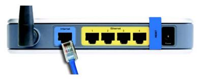
Figure 4-3: Connect the Broadband Modem
